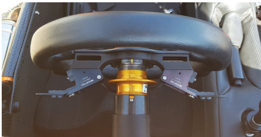
Micro switches trigger an actuator bolted to the gearbox
