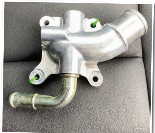
New cylinder head rear water outlet takes the existing temperature sensors for ECU and gauge (top and L) and provides a return outlet to the radiator (R) and a new outlet for the bypass hose (bottom)
