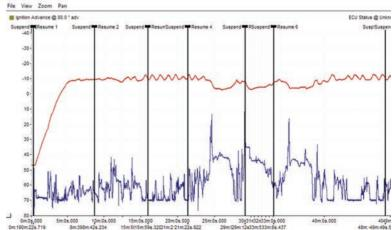
Logging throttle position (blue) and temperature (red) shows that the temperature is kept under control during both low and high-speed running
