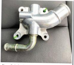
New cylinder head rear water outlet takes the existing temperature sensors for ECU and gauge (top and L) and provides a return outlet to the radiator (R) and a new outlet for the bypass hose (bottom)
