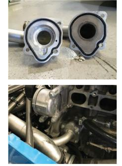
Centre: Modified water inlet (left) next to original (right). Note the cut out machined into the new backplate. Above: Partially-stripped engine bay, showing old inlet pipe still bolted to the block
