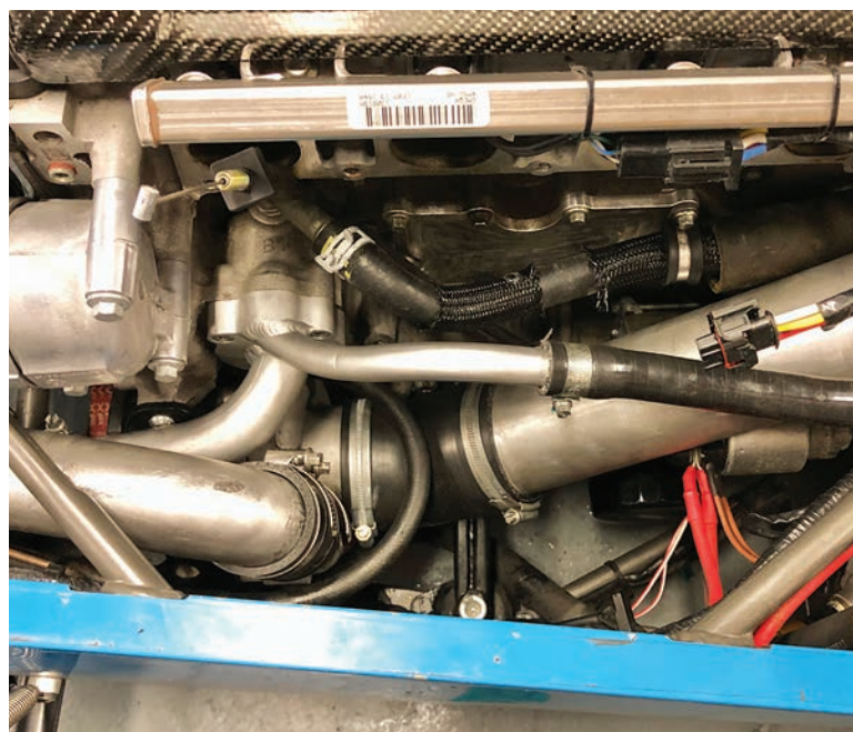
Replacement thermostat housing fitted with expansion bottle feed relocated to new spigot, ready for intercooler pipes and throttle assembly to be refitted
