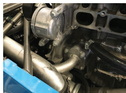
Centre: Modified water inlet (left) next to original (right). Note the cut out machined into the new backplate.
