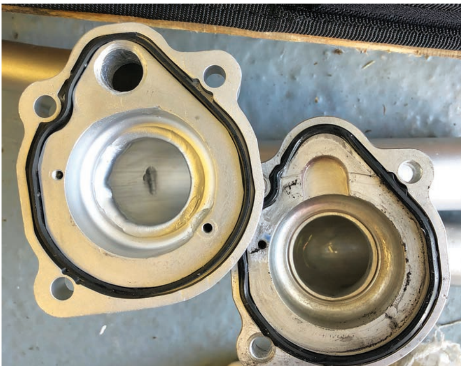
Modified housing (left) with infilled cut-out, new expansion bottle feed and additional mounting point for thermostat alongside original part
